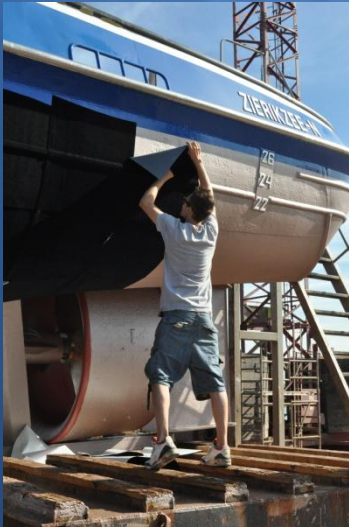
Self adhesive foil directly applied on the primer
