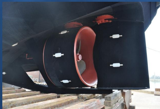
Zinc anodes are applied on top of foil
