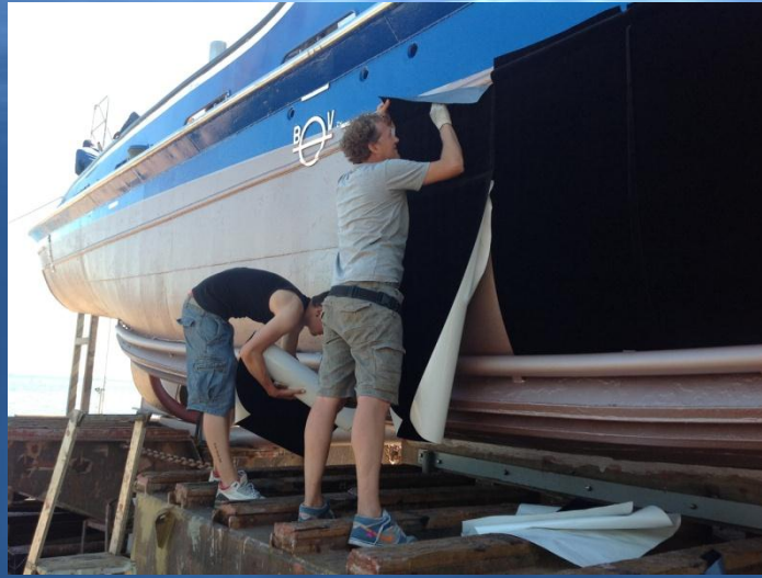
Self adhesive foil directly applied on the primer
